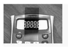
LCD with top polarizer removed from device and placed on top, such that the top and bottom polarizers are parallel.
