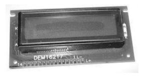
A general purpose <u>alphanumeric</u> LCD, with two lines of 16 characters. LCDs with a small number of segments, such as those used in <u>digital watches</u> and <u>pocket calculators</u>, have individual electrical contacts for each segment. A external dedicated <u>circuit</u> supplies an electric charge to control each segment. This display structure is unwieldy for more than a few display elements.
