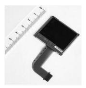
A Casio 1.8 in colour TFT liquid crystal display which equips the SonyCyber-shot DSC-P93A
